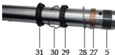
(31) CACHE POUSSIÈRE (30) CLIP (29) JOINT SPY (28) RONDELLE (27) BAGUE FIXE (5) BAGUE COULISSANTE
